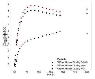
Figure 14. Approximation error for the quality of the mixture in the boiler.
