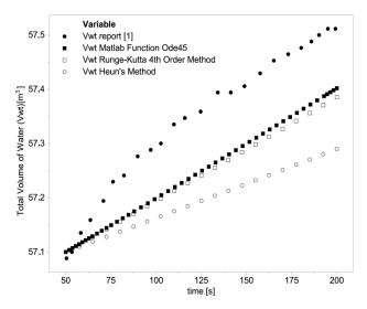
**Figure 10.** Behavior of the total volume of water with the different solution method (Ode45, Runge–Kutta, Heun).
