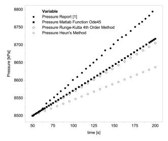
Figure 9. Pressure behavior with different solution methods (Ode45, Runge-Kutta, Heun).
