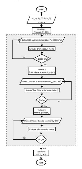
**Figure 5.** Flow chart of the code develop in MATLAB<sup>®</sup> for the Ode solution.
