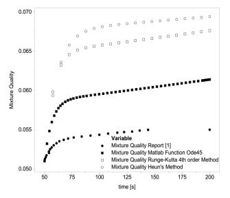
**Figure 11.** Behavior of the mixture quality with the different solution methods (Ode45, Runge–Kutta, Heun).
