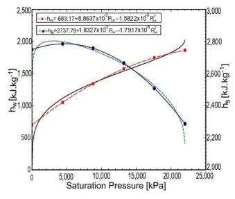
**Figure 7.** Graph used to determine the polynomials of enthalpy of water and enthalpy of steam, as a function of saturation pressure through linear regression (curve fitting) in the EES<sup>®</sup> software.
