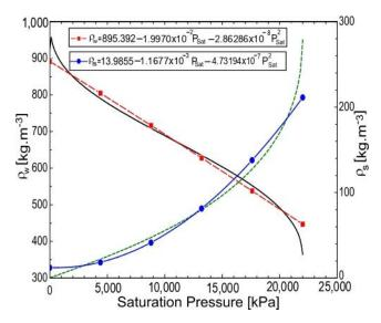
**Figure 6.** Graph used to determine the density polynomials of saturated liquid and saturated steam through linear regression (curve fitting) in the EES<sup>®</sup> software.
