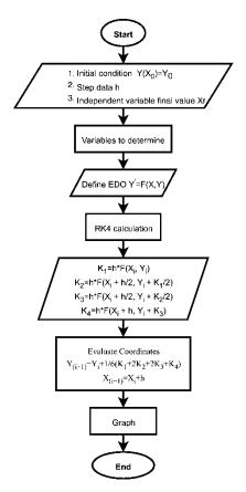
Figure 4. Flow chart of the Runge–Kutta 4th order method in MATLAB<sup>®</sup>.
