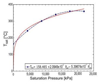
**Figure 8.** Graph used to determine the saturation temperature polynomial using linear regression (curve fitting) in the EES<sup>®</sup> software.
