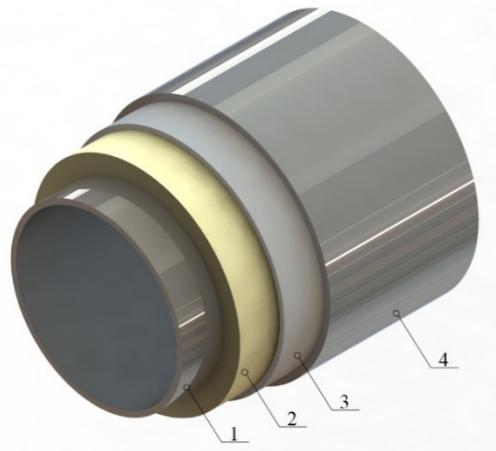
**Figure 4.** Insulating coating based on aerogel [36,38]. 1—Carrier pipe (steel ASTM 316L SS, ASTM 333 Grade 8, AISI 304); 2—A layer of insulating coating of aerogel; 3—Protective jacket pipe made of carbon steel; 4—Concrete coating.
