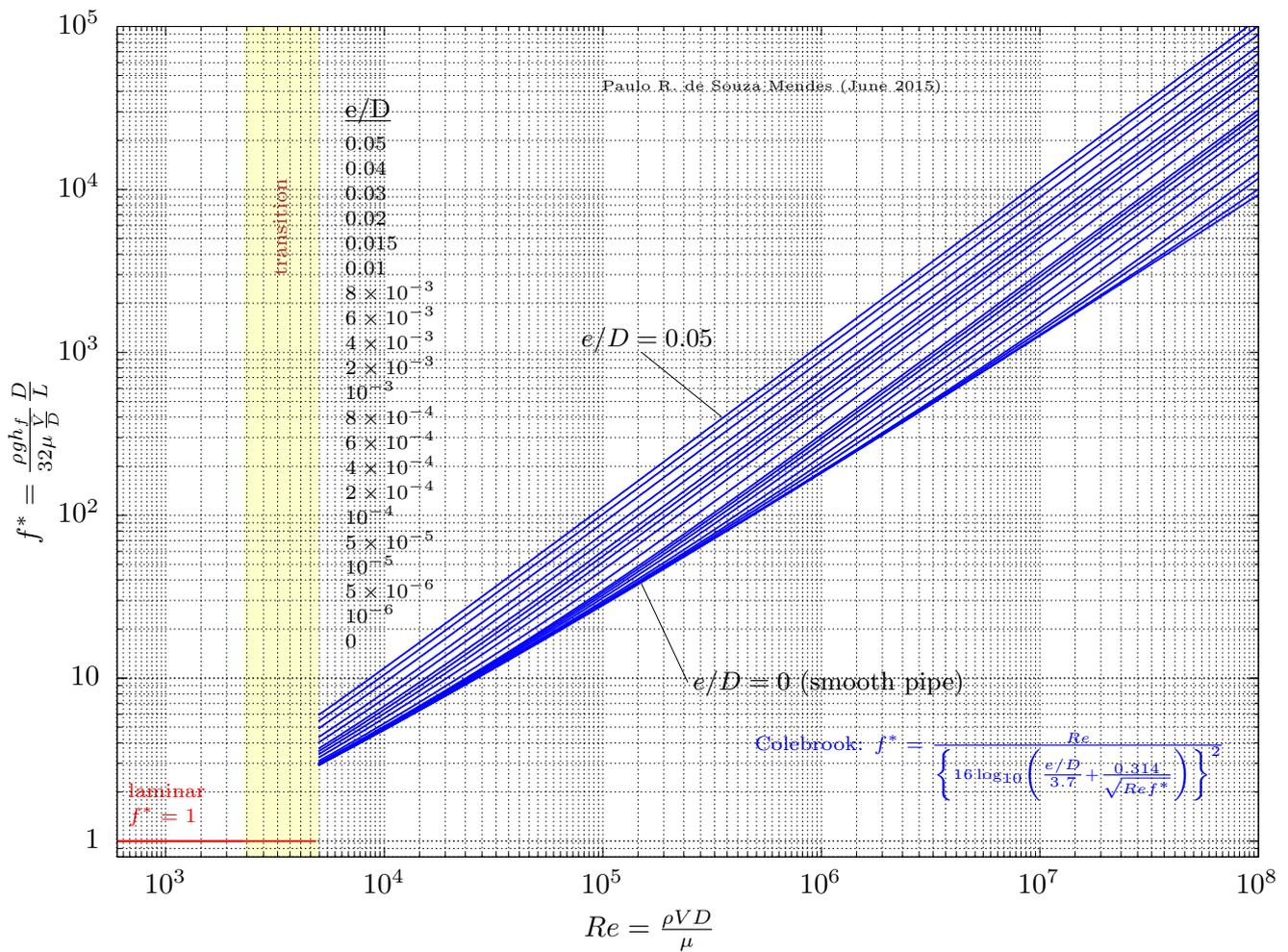
Figure 2. The modified Moody diagram.
