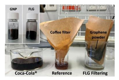
**Figure 1.** Difference in the volume occupied by 2 g of GNP and FLG powders (**upper left**); filtration setup for water purification showing a coffee filter filled with graphene powder (**right**), an empty coffee filter used for reference (**middle**) and the pure Coca-Cola<sup>®</sup> (**left**).
