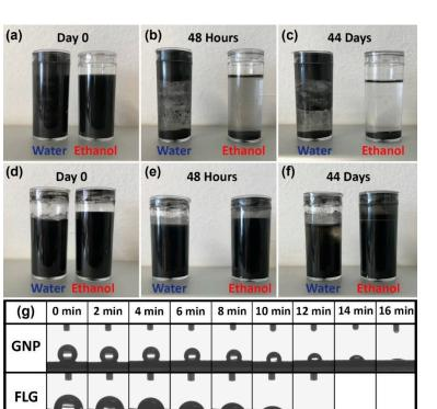
**Figure 3.** Dispersions of (a-c) GNP and (d-f) FLG powders with distilled water and ethanol directly after mixing, after 48 h and after 44 days, respectively; (g) digital pictures taken every 2 min for the water contact angle measurements of the as-prepared GNP and FLG thin films.
