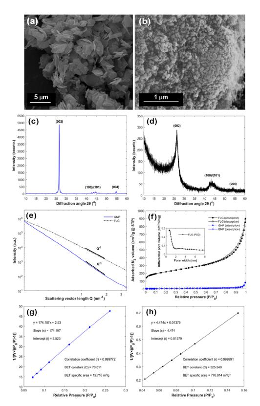
**Figure 2.** SEM images of the plasma-derived (**a**) GNP and (**b**) FLG powders, X-ray diffractograms for (**c**) GNP and (**d**) FLG, (**e**) SAXS curves, (**f**)  $N_2$  adsorption/desorption isotherms recorded at 77 K and linear multi-point BET plots for (**g**) GNP and (**h**) FLG.
