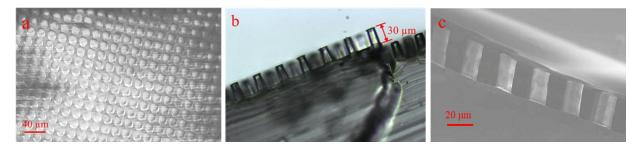
**Figure S3.** (a) SEM micrograph of PDMS substrate with the uniformly patterned array of micropillars, (b) optical image of the micropillar, c) SEM micrograph of micropillars attached on a surface
