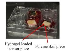
Figure S19. Photograph of the skin penetration testing used with the transdermal drug delivery system.
