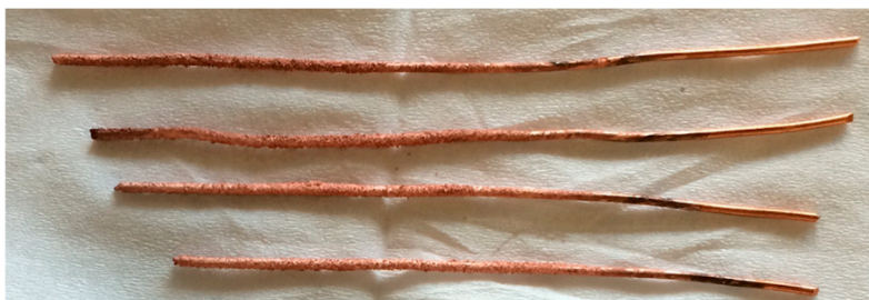
Figure 7. Examples of dried copper wire cathodes with a hard adherent Cu-SWCNT composite coating.
