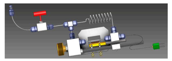
Figure 2. High-pressure sample holder used for in situ synchrotron data collection.
