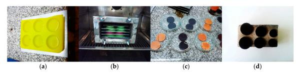
**Figure 1.** The experimental setup used for xerogel preparation: (**a**) silicon mould to keep all the disks in the same shape, (**b**) sealed chamber to avoid any solvent loss during the gelation process, (**c**) solvent exchange process, (**d**) different levels of shrinkage for carbon xerogels after pyrolysis.
