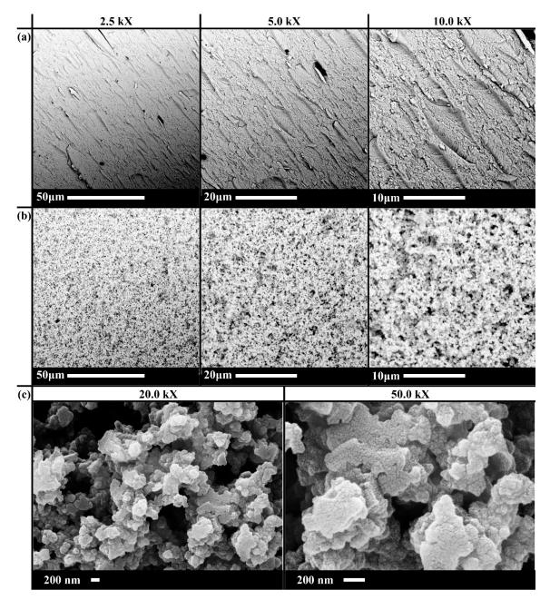
**Figure 4.** (a) SEM images of the product with maximum shrinkage (sample number 15) (b) SEM images of the product with minimum shrinkage (sample number 2). (c) FESEM images of the activated carbon xerogel at different zoom levels.
