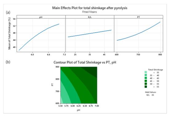
Figure 3. RSM main effect (a) and contour plots (b) for the total shrinkage of the carbon xerogel.
