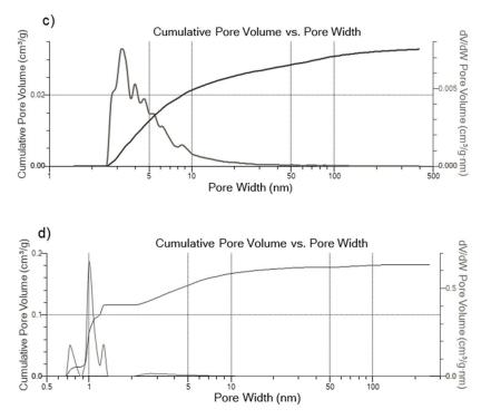
**Figure A1.** Cumulative pore volume and pore size distribution plots obtained using DFT function for (**a**) willow BC acid washed (**b**) willow AC acid washed (**c**) willow BC sulfonated (**d**) willow AC sulfonated.
