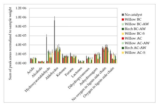
**Figure 2.** Polysaccharide and lignin pyrolysis derivatives from pine wood with and without catalytic post-treatment determined by gas chromatography with flame ionization (GC-FID). BC = biochar, AW = acid washed, S = sulfonated, AC = activated carbon.
