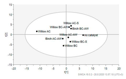
**Figure 3.** Principal component analysis (PCA) of the pyrolysis data for catalyst and no catalyst treatments (Table A1). The score plot of the two principle components shows how the samples are related to each other. BC = biochar, AW = acid washed, S = sulfonated, AC = activated carbon.
