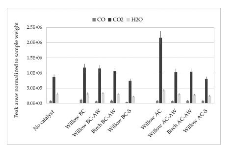
**Figure 1.** Gas and water release in thermal pyrolysis and after post-treatment. Compounds determined by GC/MSD. BC = biochar, AW = acid washed, S = sulfonated, AC = activated carbon.
