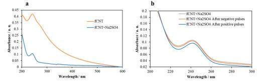
**Figure 4.** (a) UV–Vis spectra of the stable dispersion of *f*CNTs (orange line) and *f*CNTs + 0.1 M Na<sub>2</sub>SO<sub>4</sub> (blue line). (b) UV–Vis spectra of the stable dispersion of *f*CNTs + 0.1 M Na<sub>2</sub>SO<sub>4</sub> (grey line) after negative (orange line) and positive pulses (blue line).
