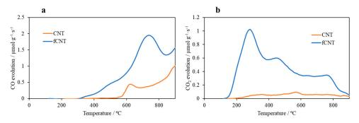
Figure 3. (a) CO<sub>-</sub> and (b) CO<sub>2</sub>\_TPD evolution profiles for CNT (orange lines) and *f*CNT (blue lines) samples.
