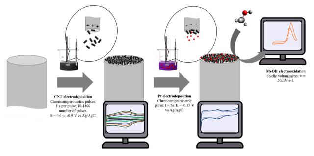
Figure 1. Schematic representation of the experimental procedure used in this work.
