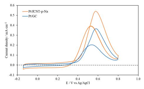
**Figure 10.** Cyclic voltammograms of Pt/*f*CNT-p-Na (orange line) and Pt/GC (blue line) in a 0.1 M MeOH + 0.5 M H<sub>2</sub>SO<sub>4</sub> solution. Scan rate = 50 mV s<sup>-1</sup>.
