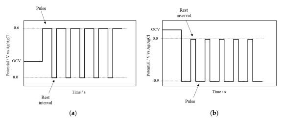
**Figure 2.** Scheme of the potential step of multiple steps during the electrochemically assisted deposition of *f*CNTs at (**a**) positive and (**b**) negative potentials.
