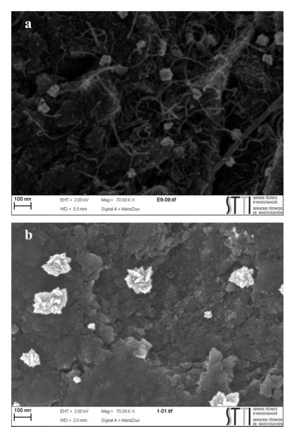
**Figure 9.** FESEM images of (**a**) Pt/*f*CNT-p-Na and (**b**) Pt/GC.
