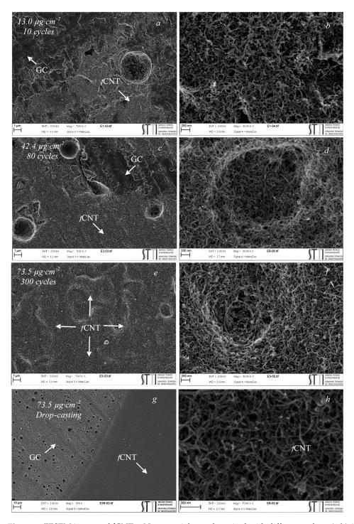
**Figure 7.** FESEM images of *f*CNT-p-Na potential step deposited with different pulses: (**a**,**b**) 10, (**c**,**d**) 80, and (**e**,**f**) 300 pulses. (**g**,**h**) FESEM images of *f*CNTs deposited via drop-casting with the same *f*CNT loading as that shown in (**e**).
