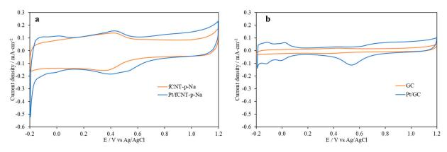
**Figure 8.** Cyclic voltammograms before and after the electrodeposition of platinum nanoparticles on (**a**) *f*CNT-p-Na (orange line) and Pt/*f*CNT-p-Na (blue line) electrodes and (**b**) GC (orange line) and Pt/GC (blue line) electrodes; 0.5M H<sub>2</sub>SO<sub>4</sub>,  $v = 50 \text{ mV s}^{-1}$ .
