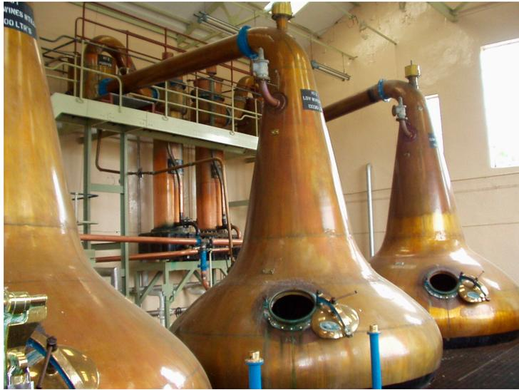
**Figure 22.** A typical pot still employed for the batch distillation of malt whisky.
