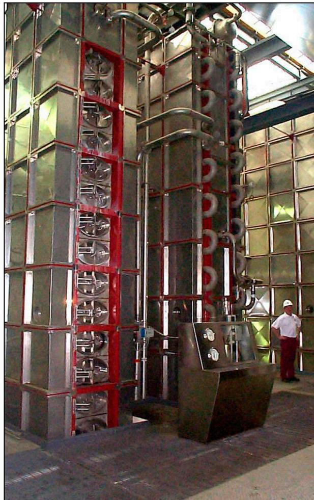
**Figure 23.** Coffey still employed for the continuous distillation of grain whisky.
