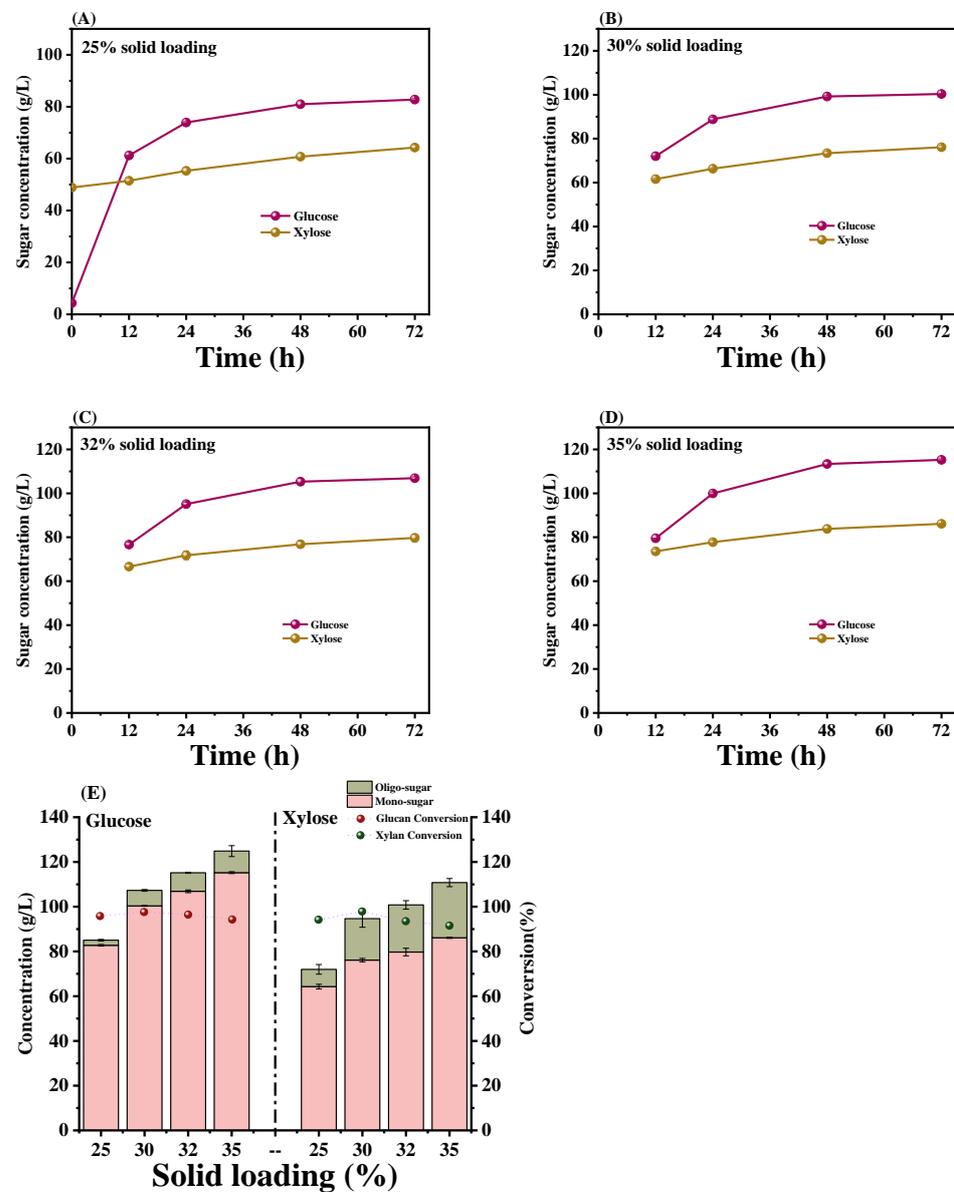
Figure 3. Enzymatic hydrolysis of DLCA(sa)-CC at 25% (A), 30% (B), 32% (C), and 35% (D) solid loading and sugar conversions at different solids loadings (E). Enzymatic hydrolyses were performed at 50 °C, 250 rpm, and pH 4.8 with an enzyme dosage of 15 mg protein/g glucan.
