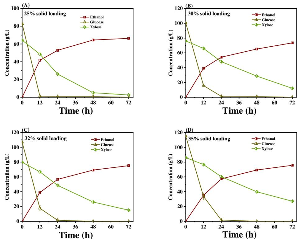
**Figure 4.** Ethanol fermentation in hydrolysates of DLCA(sa)-CC at 25% (A), 30% (B), 32% (C), and 35% (D) solid loading. *S. cerevisiae* CRD5HS (initial  $OD_{600} = 2$ ) was used for fermentation at pH 5.5, 30 °C, 150 rpm for 72 h.
