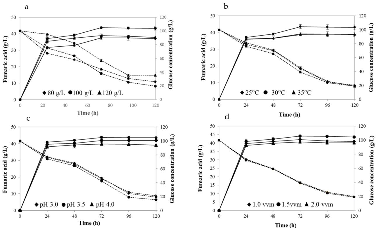
**Figure 1.** Fumaric acid concentration (solid line) and remaining glucose (dash line) at various initial glucose concentrations (g/L) (a), temperature (b), pH (c), and aeration rate (d).
