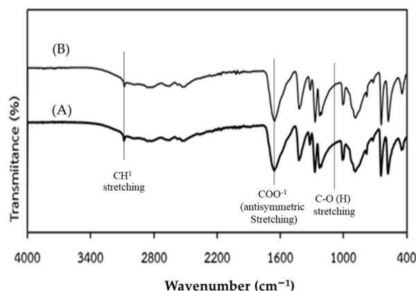
**Figure 3.** FTIR spectra of (A) commercial fumaric acid (FA) and (B) biosynthesized FA measured in the range of 4000–400  $\text{cm}^{-1}$  with a resolution of 4  $\text{cm}^{-1}$  and 32 scans.
