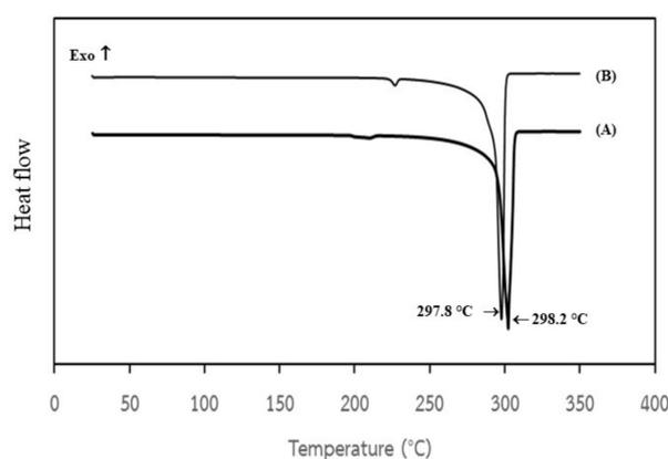
**Figure 4.** DSC scans of (A) commercial fumaric acid (FA) and (B) bio-synthesized FA.
