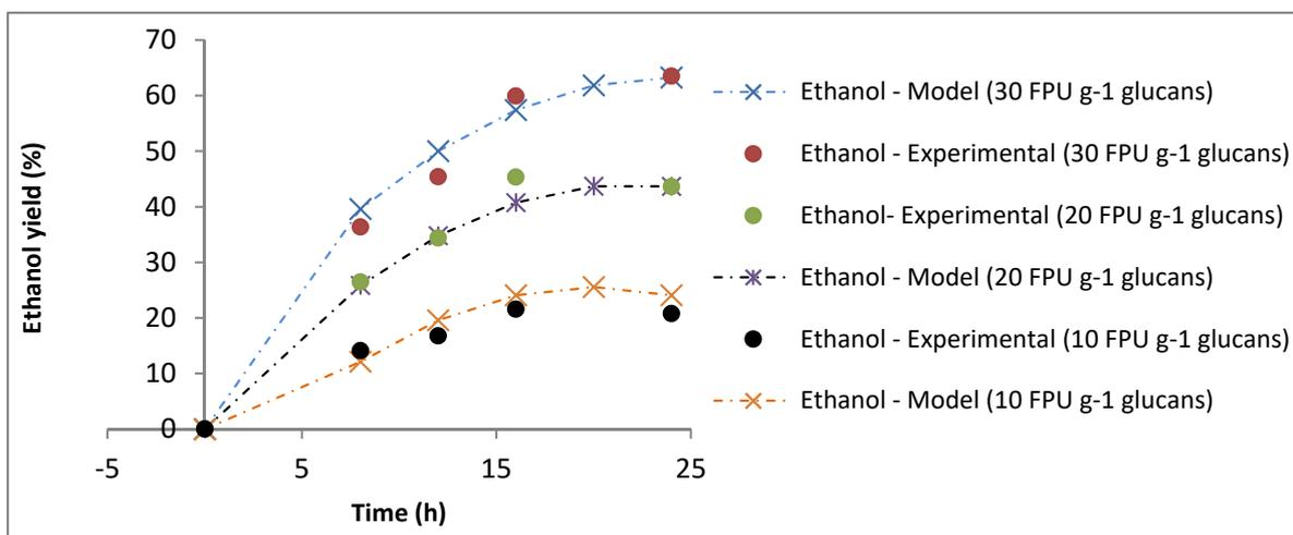
Figure 3. Experimental and theoretical (calculated using Model I) fermentation yields at 39 °C.
