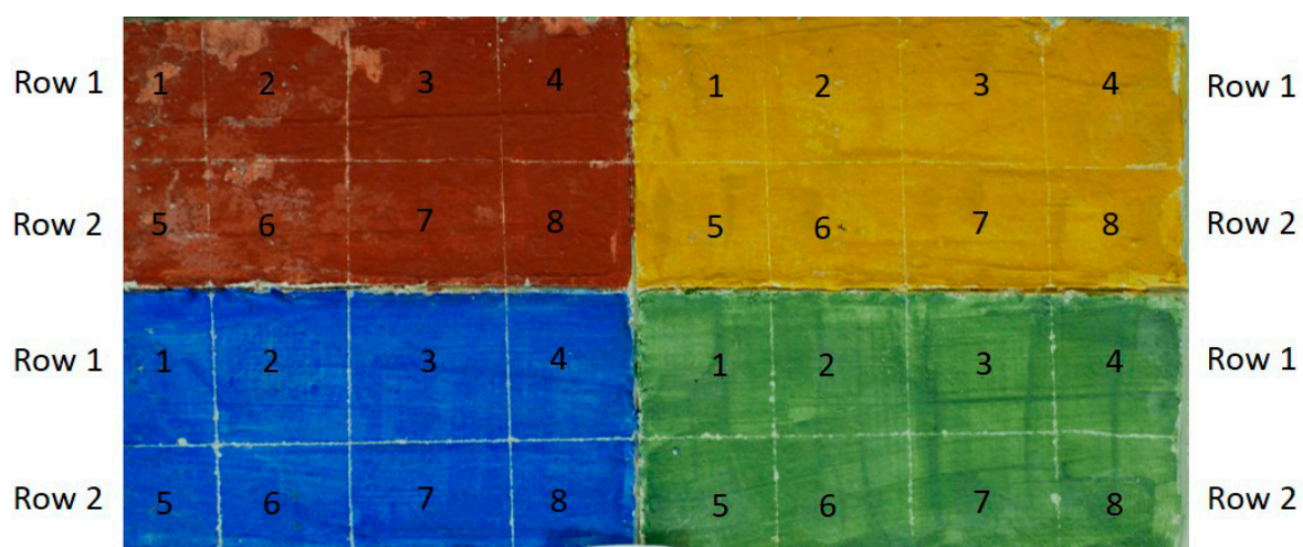
Figure S1. Painted laboratory models divided in squares for inoculation of fungi. Row 1.1 and Row 2.5 - inoculation with Penicillium sp. BSL3-2; Row 1.2 and Row 2.6 - inoculation with Aspergillus sp. BSL 2-2; Row 1.3 and Row 2.7 - inoculation with Emericellopsis sp. MM2; Row 1.4 and Row 2.8 - inoculation with strain H1.
