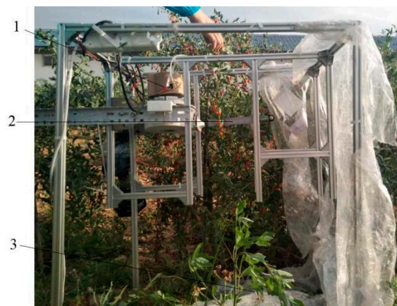
Figure 7. Chinese wolfberry harvesting performance test: 1. Chinese wolfberry harvesting test platform. 2. electronic angle ruler. 3. fruit collection cloth.
