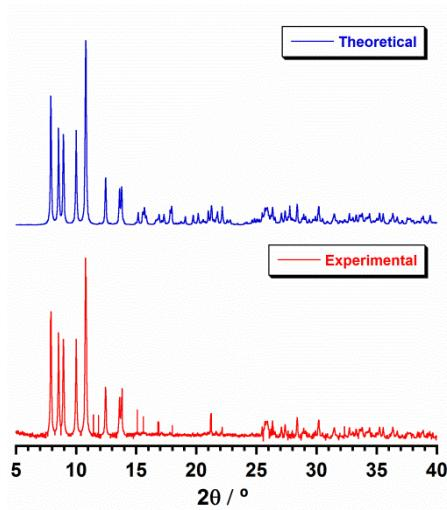
**Figure S2.** Plots of the theoretical and experimental XRD patterns profile ( $2\theta/\text{°}$ ) in the range  $5\text{-}40\text{°}$  for compounds **1** (top) and **2** (bottom).
