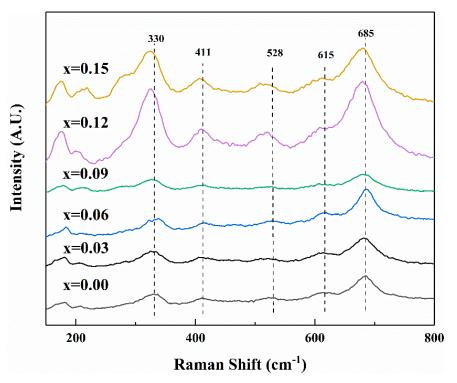
Figure 5. Raman spectra of the  $SrFe_{12-x}Nb_xO_{19}$  (x = 0.00-0.15) powders.
