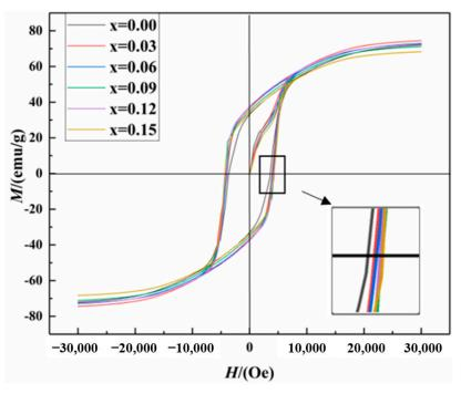
**Figure 8.** Magnetic hysteresis loops of  $SrNb_xFe_{12-x}O_{19}$  (x = 0.00-0.15) hexaferrites.
