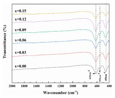
**Figure 4.** FTIR spectra of  $SrFe_{12-x}Nb_xO_{19}$  (x = 0.00–0.15) hexaferrites.
