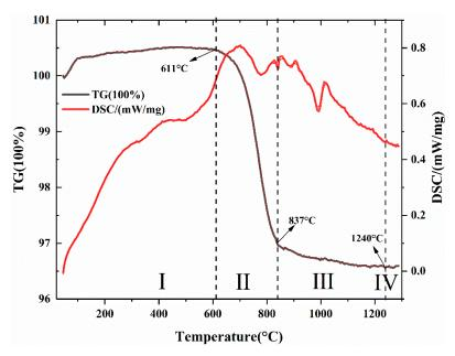
**Figure 1.** TG/DSC scanning curve for SrFe<sub>12</sub>O<sub>19</sub>.
