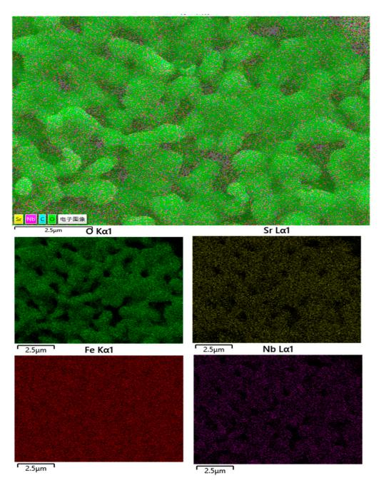
**Figure 7.** Elemental mapping results for  $SrFe_{12-x}Nb_xO_{19}$  (x = 0.09) hexaferrites.
