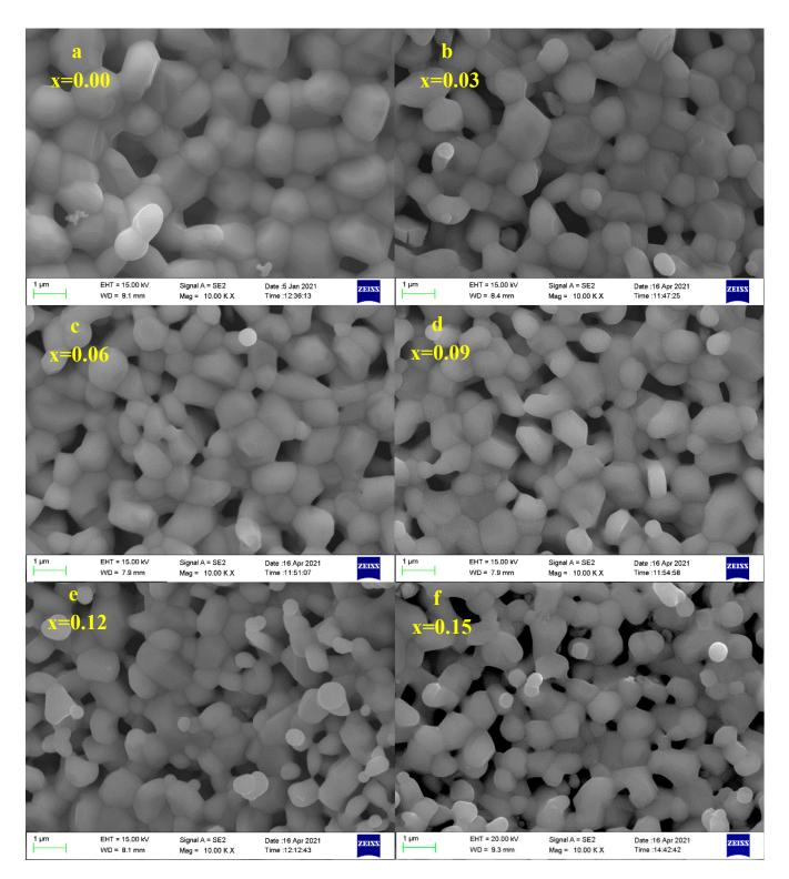
**Figure 6.** SEM micrographs of  $SrFe_{12-x}Nb_xO_{19}$  (x = 0.00–0.15) hexaferrites. (**a**) x = 0.00; (**b**) x = 0.03; (**c**) x = 0.06; (**d**) x = 0.09; (**e**) x = 0.12; (**f**) x = 0.15.
