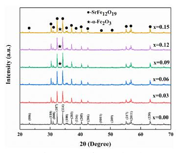
**Figure 2.** Powder XRD patterns of  $SrFe_{12-x}Nb_xO_{19}$  (0.00  $\leq x \leq$  0.05) HFs.
