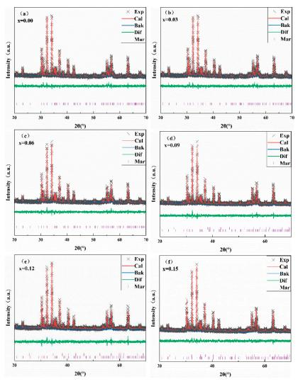
**Figure 3.** Rietveld refined power XRD patterns for all Nb substituted hexaferrites. (a) x = 0.00; (b) x = 0.03; (c) x = 0.06; (d) x = 0.09; (e) x = 0.12; (f) x = 0.15.
