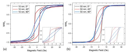
**Figure 2.** Room temperature hysteresis loops recorded from (**a**) 10 nm thick and (**b**) 50 nm thick permalloy thin films grown using electron-beam evaporation with an applied field of 500 Oe. The angles indicated in the legend correspond to the field direction with respect to the applied field during growth. Insets are zoomed regions around  $H_C$  for each plot.
