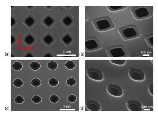
**Figure 1.** SEM images of the antidot lattices studied, including the 10 nm thick antidot lattices (a,b) and the 50 nm thick antidot lattices (c,d). Panels (b,d) are tilted SEM images taken at an angle of 30 degrees with respect to the electron beam direction. The red arrows denote the directions along which the hysteresis loops are measured. The direction of the applied field during growth corresponded to  $0^{\circ}$ .
