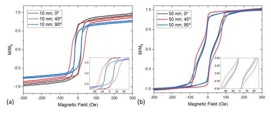
**Figure 3.** Room temperature hysteresis loops recorded from (**a**) 10 nm thick and (**b**) 50 nm thick permalloy antidot lattices grown by electron-beam evaporation with an applied field of 500 Oe parallel to one lattice axis ( $0^\circ$ ). Insets are zoomed regions around Hc for each plot.
