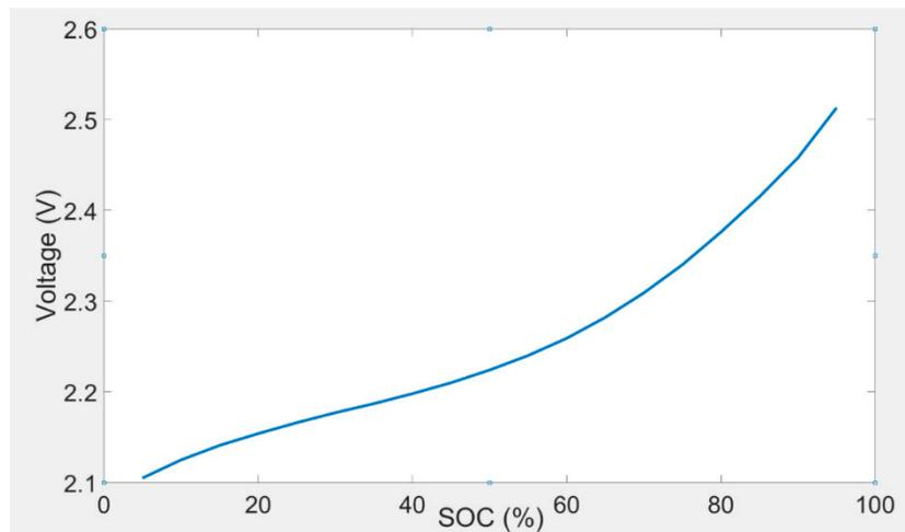
**Figure 2.** OCV and SOC characteristic at 30 °C.
