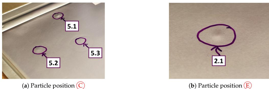
**Figure 11.** External in-situ visibility of particles found in Figures 7a and 5b dependent of depth in cell layers and particle size (Particle 5.1 > 5.2 > 5.3).
