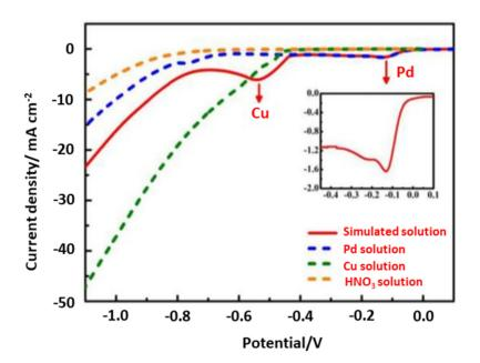
**Figure 4.** The linear sweep voltammogram (LSV) curves of the simulated solution, a Pd<sup>2+</sup> solution, Ca u<sup>2+</sup> solution, and HNO<sub>3</sub>. Reproduced with permission [62]. Copyright 2020, Elsevier.
