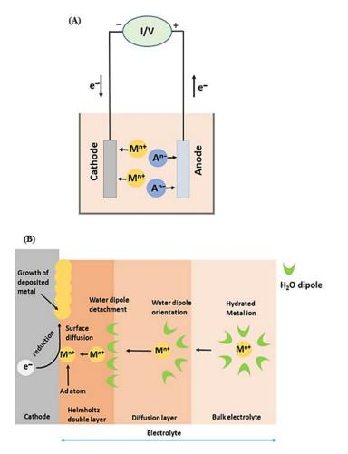
Figure 2. Schematic representation of electrodeposition process (A) and mechanism details (B).
