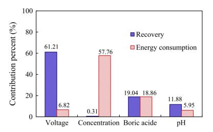
**Figure 5.** The contribution percent of the parameters (voltage, concentration, boric acid, and pH) of electrodeposition on Ni recovery and energy consumption. Reproduced with permission [68]. Copyright 2014, Elsevier.
