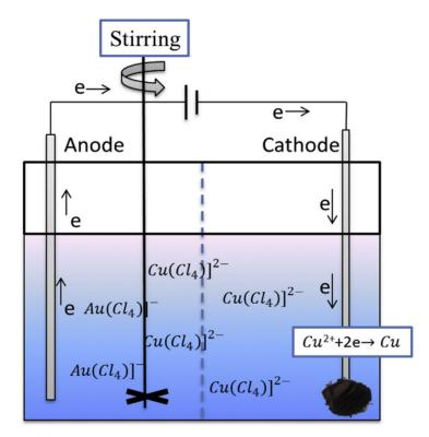
**Figure 11.** Schematic diagram of the electrodeposition process in HCl-NaCl-H<sub>2</sub>O<sub>2</sub> system. Reproduced with permission [81]. Copyright 2019, Elsevier.
