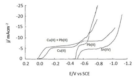
**Figure 10.** The LSV curves for 0.01 M Cu(NO<sub>3</sub>)<sub>2</sub> + 0.5 M NaNO<sub>3</sub>, 0.01 M Pb(NO<sub>3</sub>)<sub>2</sub> + 0.5 M NaNO<sub>3</sub>, 0.01 M Cu(NO<sub>3</sub>)<sub>2</sub> + 0.01 M Pb(NO<sub>3</sub>)<sub>2</sub> + 0.5 M NaNO<sub>3</sub>, 0.01 M H<sub>2</sub>SnCl<sub>6</sub> + 1.5 M HCl at a scan rate of 5 mV s<sup>-1</sup>. Reproduced with permission. [88] Copyright 2002, Wiley.
