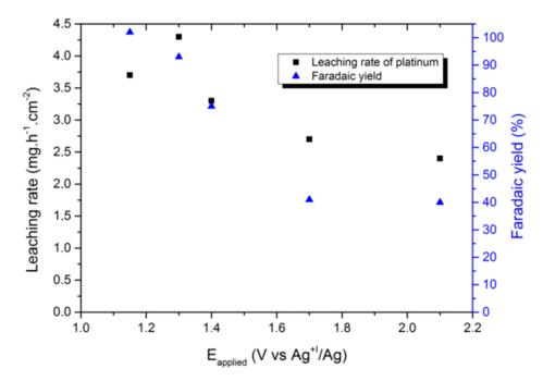
**Figure 12.** Effect of the applied potential on the leaching rate of platinum and the corresponding Faradaic yield in runs conducted at  $Q = 55 \text{ C} \cdot \text{cm}^{-2}$ . Reproduced with permission [89]. Copyright 2018, Creative Commons.
