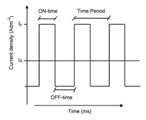
**Figure 6.** The typical pulse–current waveform showing T<sub>on</sub> and T<sub>off</sub> for one cycle. Reproduced with permission [70]. Copyright 2008, Elsevier.
