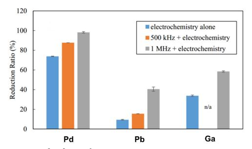
**Figure 9.** Reduction ratio of Pd<sup>2+</sup>, Pb<sup>2+</sup>, and Ga<sup>3+</sup> metal ions over 60 min in Ar-saturated solution (with or without 500 kHz or 1 MHz sonication). Reproduced with permission [83]. Copyright 2016, Elsevier.
