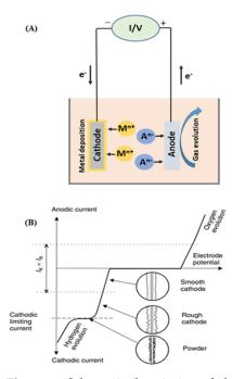
**Figure 7.** Schematic description of electrowinning process (**A**) and current density–cell voltage dependence for the electrowinning of copper (**B**). Reproduced with permission [16]. Copyright 2007, Wiley.
