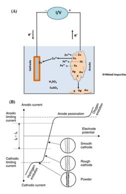
**Figure 8.** Schematic description of electrorefining process (**A**) and current density–cell voltage dependence for the electrorefining of copper (**B**). Reproduced with permission [16]. Copyright 2007, Wiley.
