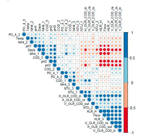
**Figure 3.** Correlation matrix between different quali-quantitative parameters of the multistage system treating greywater. The red and blue dots correspond to negative and positive correlations, respectively. Small dots with light colors represent lower intensity correlations, and larger dots with darker colors correspond to higher intensity correlations.
