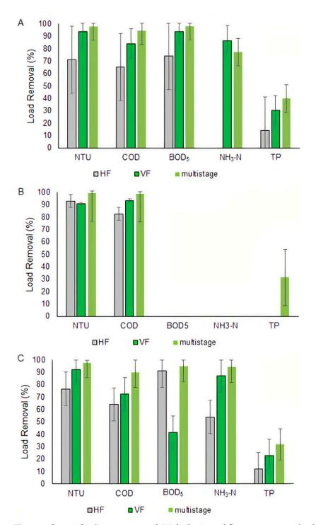
**Figure 2.** Organic loading rate removal (%) for horizontal flow treatment wetland (HF-CW), vertical flow treatment wetland (VF-CW), and CW system at phase 1 (**A**), 2 (**B**), and 3 (**C**). NTU (turbidity); COD (chemical oxygen demand); BOD (biochemical oxygen demand); NH<sub>4</sub><sup>+</sup> (ammonia); and TP (total phosphorous).
