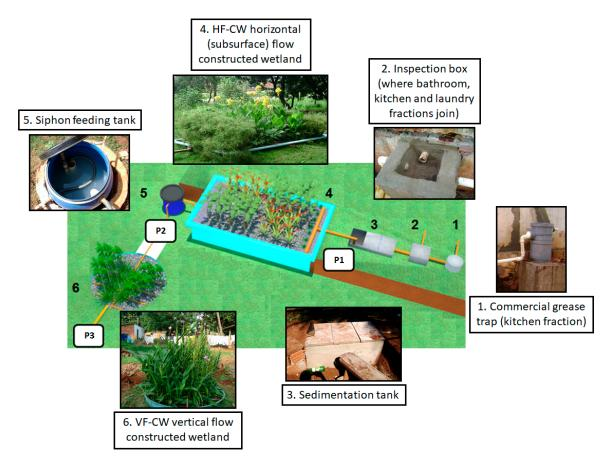
Figure 1. Set up of the constructed wetland (CW) system representing the pre-treatment and multistage system.
