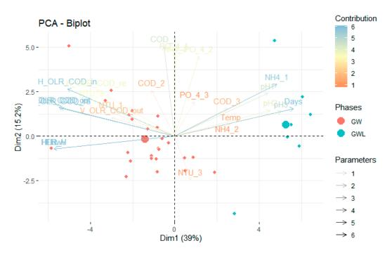
**Figure 4.** Principal component analysis (PCA) in greywater with (GW) and without kitchen sink component ( $GW_L$ ) treated by constructed wetlands (multistage system). Contributions of quali-quantitative parameters by PCA with cluster (GW and  $GW_L$ ).
