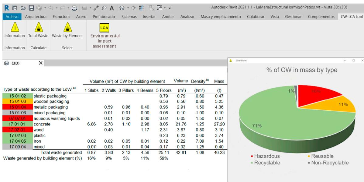
**Figure 2.** Identification and quantification of recyclable CW fractions. <sup>a)</sup> European List of Waste [48]; <sup>b)</sup> National Ratios Generation of Waste Study from Construction and Demolition [49].
