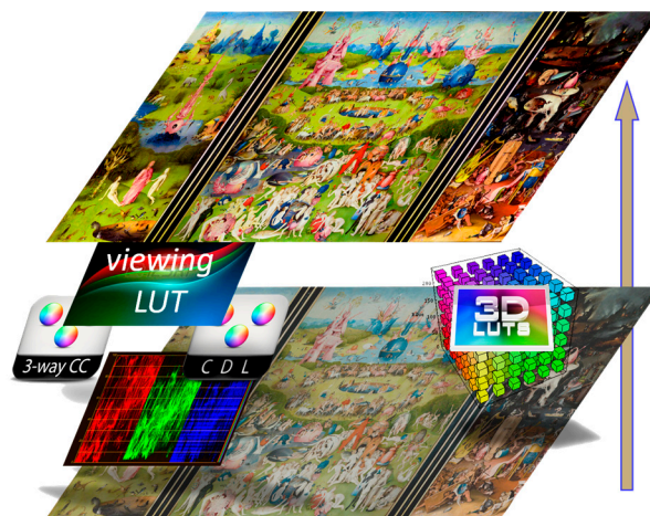
Figure 3. Toy-model of a simple, single-camera, non-ACES “basic” grading pipeline: the arrow on the right orders the “layer-based” representation of real-time image processing operations, as performed by the color-correction system in the background, while colorist works. Source footage in its camera-native colorimetry ( bottom ) is creatively modified by color transforms, either coming from the set (Color Decision Lists, cfr. Section 2.4) and applied in-theater (3-way CC’S); then a “viewing LUT” is applied on top to match the colorimetry with the output device’s for viewing ( top ). A 3D LUT may represent the overall effect of a single primary grade (possibly lacking accuracy [17,20]), and may include the viewing LUT and all color-space conversions (courtesy: Hieronymus Bosch, The Garden of Earthly Delights , c.1495–1505).
