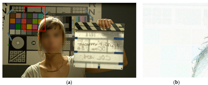
Figure 16. Camera-department tests: (a) camera-test footage, as processed by on-set equipment (no CDL), with detail zone in red; (b) differences with the same footage and same processing by finishing department (white areas mean the two sources sum to 0). High-frequency discrepancies are evident.
