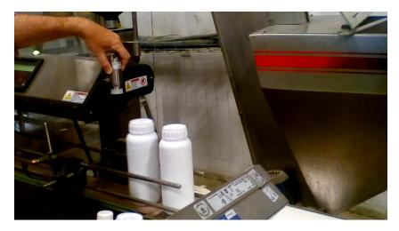
**Figure 13.** Picture taken in the production line during a stop. It shows two bottles right after they passed below the thermal camera. The human hand is adjusting the thermal camera.
