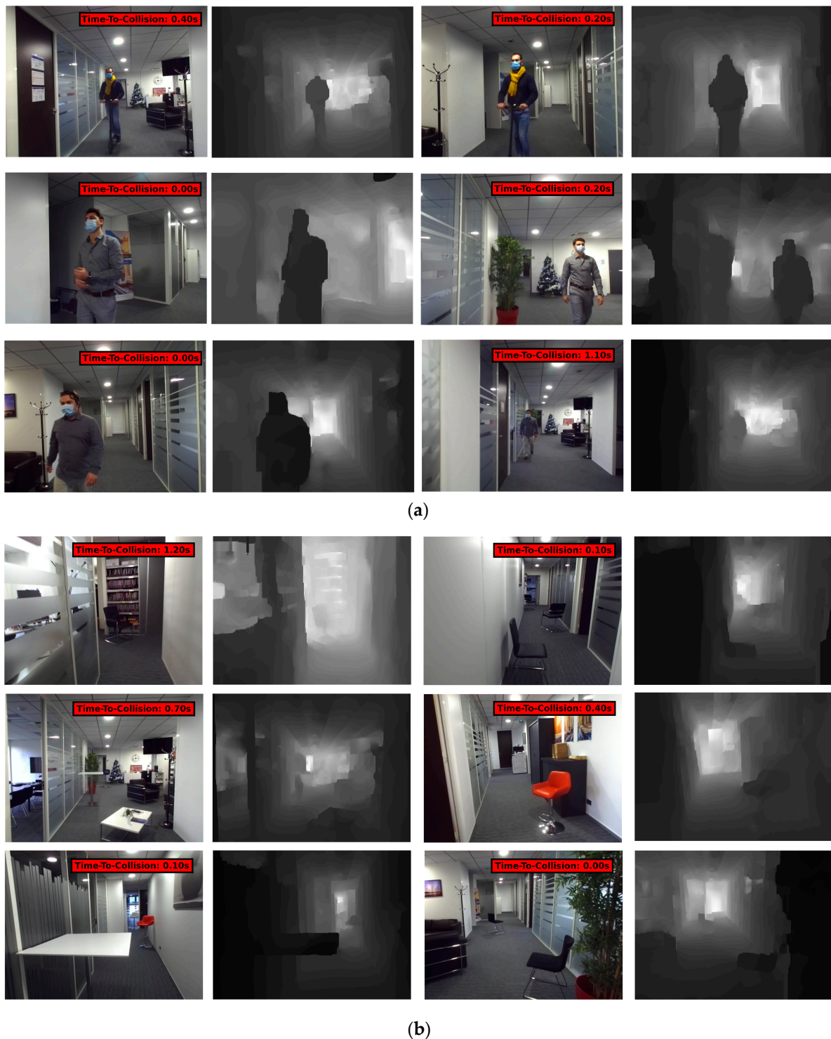
Figure 7. Our dataset used for testing purpose. Color RGB frames with labeled Time-to-Collision and corresponding depth maps. (a) Videos with only dynamic obstacles (pedestrians and scooter); (b) videos with only static obstacles on the path (chairs and desks).
