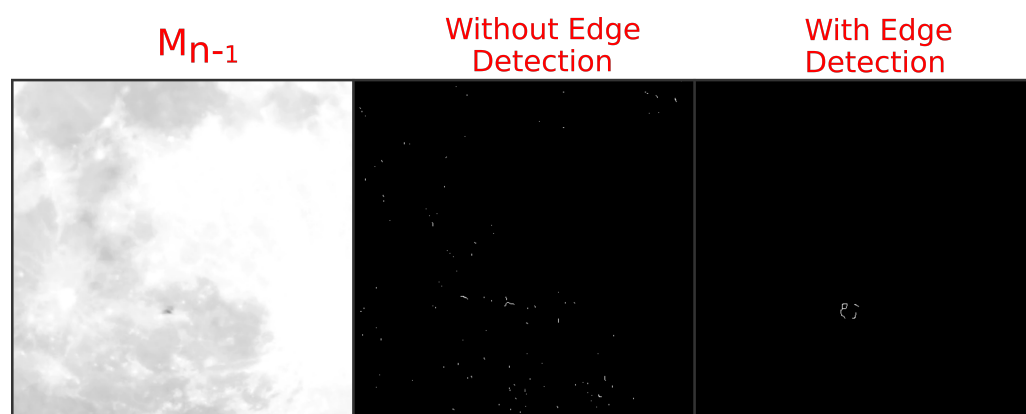
Figure 4. Performing edge detection is necessary for object detection on a complicated background. The image of the bird silhouette in front of the moon in the original image has been processed through the UnCanny detector without and with the Sobel edge detection steps. Excluding edge detection from the process produces an image with many errors generated by slight differences in the background between input images M_{n-1} and M_n .
