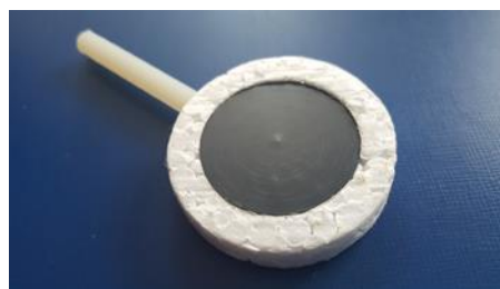
Figure 2. Photo of a polyvinyl chloride (PVC) sample with sample holder.
