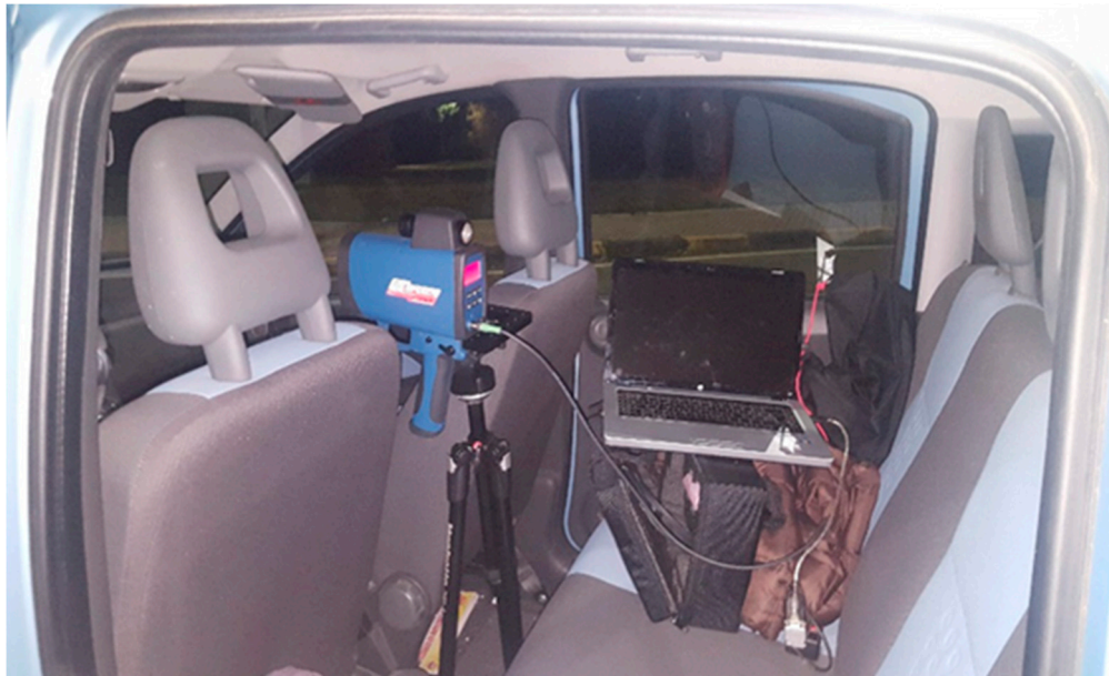
Figure 2. Speed data collection with the telelaser hidden in the car.
