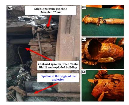
**Figure 3.** (a) Confined space below the ground surface and (**b**–**d**) different views of the corroded pipe (Recreated after [21]).
