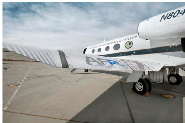
**Figure 6.** Adaptive Compliant Trailing Edge (ACTE) flaps on NASA's Gulfstream III aeronautical test bed [13].
