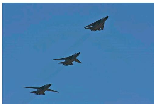
**Figure 3.** F-111 Aircraft wing sweep modification sequence [5].
