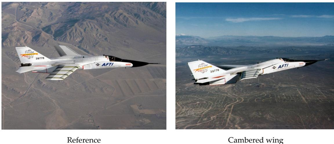
**Figure 4.** AFTI/F-111 aircraft in flight [7,8] with a variable camber wing.
