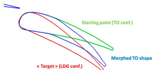
**Figure 19.** Application of morphing technology on the flap system.
