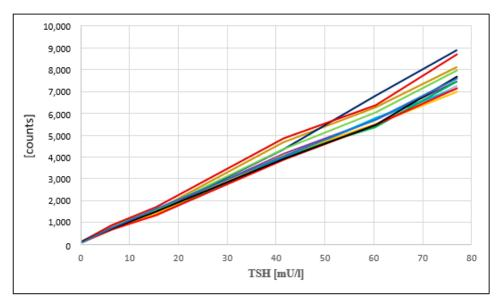
Figure 4. Calibration curves of 12 measurements with the Labsystems/NS2400 over 5 weeks.
