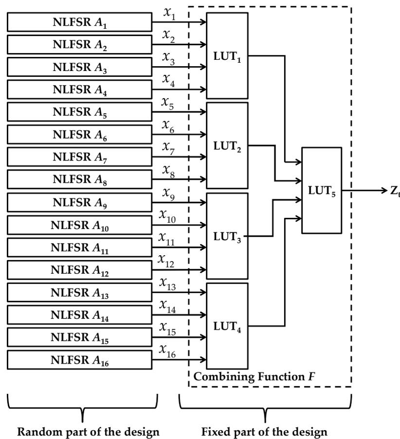
Figure 4. Description of the created keystream generator.
