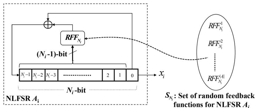
Figure 5. General structure of the selected NLFSRs sets.
