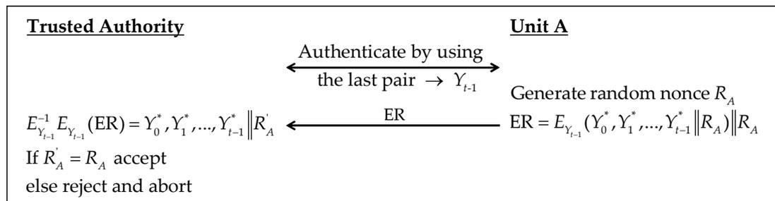
Figure 7. Update protocol of SUC based on random stream cipher.
