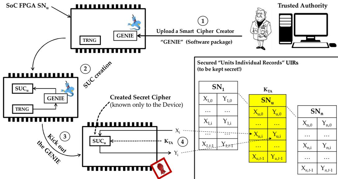
Figure 1. The concept for creating SUCs in SoC FPGAs environment.
