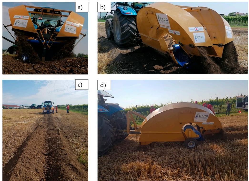
**Figure 2.** Views of (a) the rear of the prototype, where the iron triangle shaped structure is partially visible behind the removable impermeable film, (b) the soil being discharged on the film, (c) the appearance the SWRS at the end, and (d) a lateral view of the prototype.
