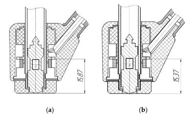
**Figure 4.** The position of the induction coil relative to the surface of test piece for standard (**a**) and modified (**b**) type D impact device.
