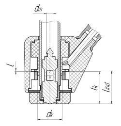
Figure 3. The location of the impact body relative to the induction coil at the time of indentation.
