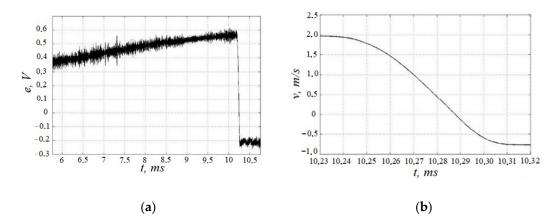
**Figure 6.** Graph of EMF e(t) induced on the induction coil during measurement (**a**) and graph of the impact body velocity during the indentation process (**b**).
