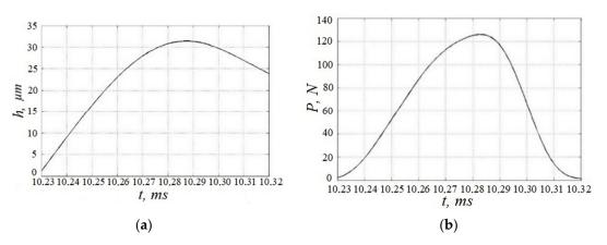
**Figure 7.** Graphs of the depth of penetration across time (**a**) and the graph of the applied load across time (**b**).
