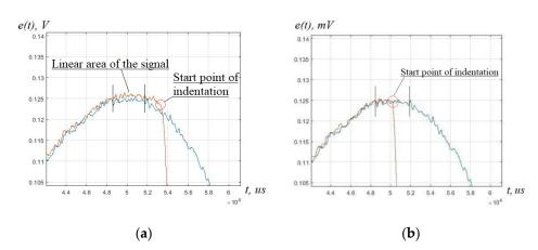
Figure 5. Signal obtained using a standardized (a) and modified (b) Leeb D impact device.
