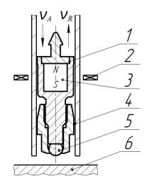
**Figure 1.** Leeb hardness measuring scheme: 1—impact body, 2—induction coil, 3—magnet, 4—guiding tube; 5—indenter; 6—test piece.
