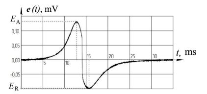
Figure 2. Graph of EMF *e*(*t*), induced in induction coil during measurement.
