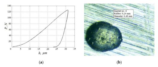
Figure 8. Load–displacement diagram (a) and photograph of the indentation (b).
