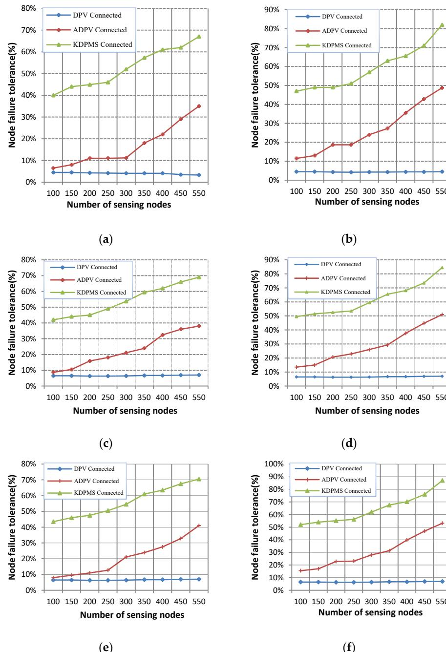
**Figure 4.** Percentage of failed nodes when supernode disconnectivity occurs: (a)  $k = 2$ ,  $S_r = 3\%$ , (b)  $k = 2$ ,  $S_r = 5\%$ , (c)  $k = 3$ ,  $S_r = 3\%$ , (d)  $k = 3$ ,  $S_r = 5\%$ , (e)  $k = 4$ ,  $S_r = 3\%$ , and (f)  $k = 5$ ,  $S_r = 5\%$ .
