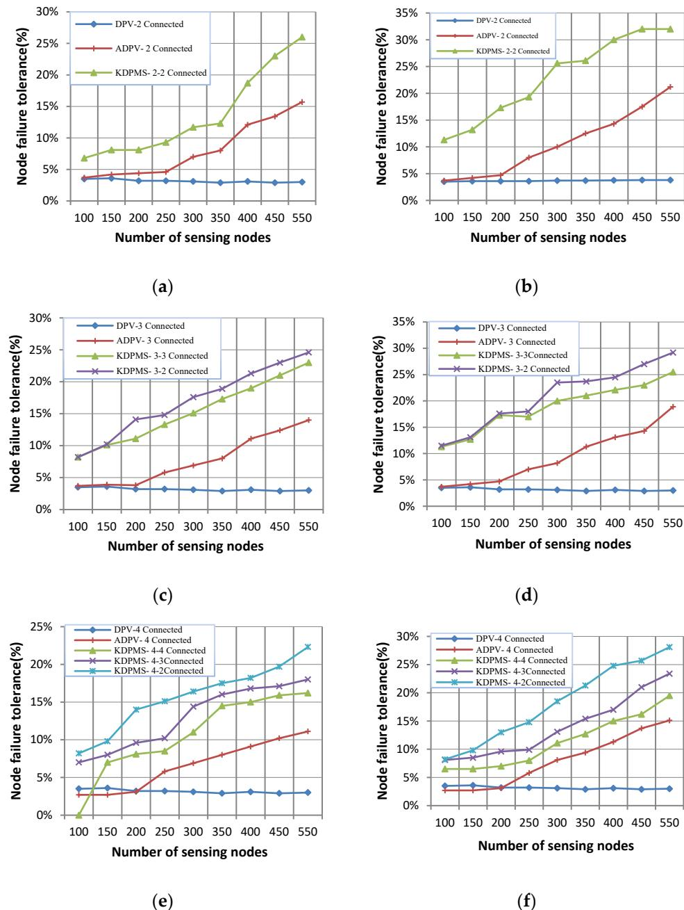
**Figure 5.** Percentage of failed nodes when  $k$ -vetrrex supernode disconnectivity occurs: (a)  $k = 2$ ,  $Sr = 3\%$ , (b)  $k = 2$ ,  $Sr = 5\%$ , (c)  $k = 3$ ,  $Sr = 3\%$ , (d)  $k = 3$ ,  $Sr = 5\%$ , (e)  $k = 4$ ,  $Sr = 3\%$ , and (f)  $k = 5$ ,  $Sr = 5\%$ .
