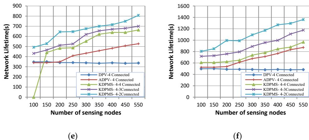
**Figure 7.** Comparison of  $k$ -vertex supernode connectivity lifetime in DPV, ADPV and KDPMS: (a)  $k = 2$ ,  $Sr = 3\%$ , (b)  $k = 2$ ,  $Sr = 5\%$ , (c)  $k = 3$ ,  $Sr = 3\%$ , (d)  $k = 3$ ,  $Sr = 5\%$ , (e)  $k = 4$ ,  $Sr = 3\%$ , and (f)  $k = 5$ ,  $Sr = 5\%$ .
