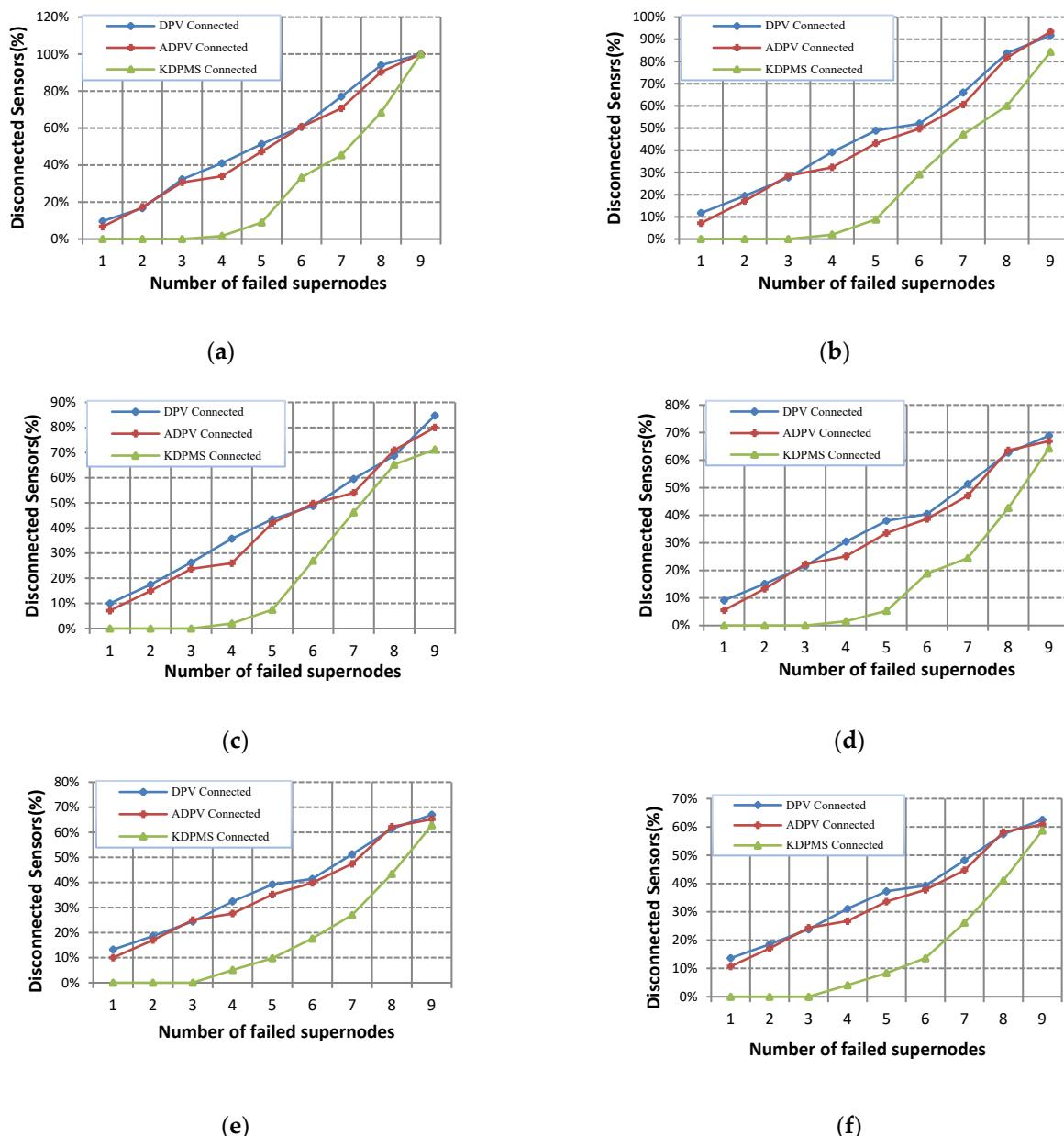
**Figure 8.** Comparison of supernode failure tolerance in DPV, ADPV, and KDPMS: (a)  $N = 300$ , (b)  $N = 350$ , (c)  $N = 400$ , (d)  $N = 450$ , (e)  $N = 500$ , and (f)  $N = 550$ .
