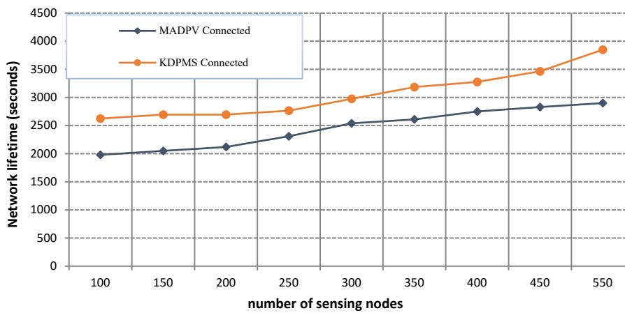
**Figure 11.** Lifetime comparison of the KDPMS and MADPV algorithms.
