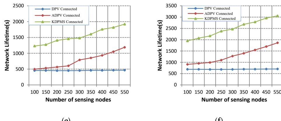
**Figure 6.** Comparison of supernode connectivity lifetime in DPV, ADPV and KDPMS: (a)  $k = 2$ ,  $S_r = 3\%$ , (b)  $k = 2$ ,  $S_r = 5\%$ , (c)  $k = 3$ ,  $S_r = 3\%$ , (d)  $k = 3$ ,  $S_r = 5\%$ , (e)  $k = 4$ ,  $S_r = 3\%$ , and (f)  $k = 5$ ,  $S_r = 5\%$ .
