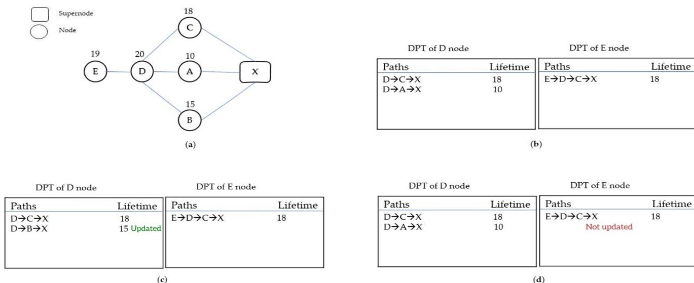
**Figure 3.** Redundant control message: (a) initial topology, (b) disjoint paths of nodes D and E, (c) disjoint paths of nodes D and E after the pathinfo message has been sent by node B, and (d) disjoint paths of nodes D and E after the pathinfo message has been sent by node D.
