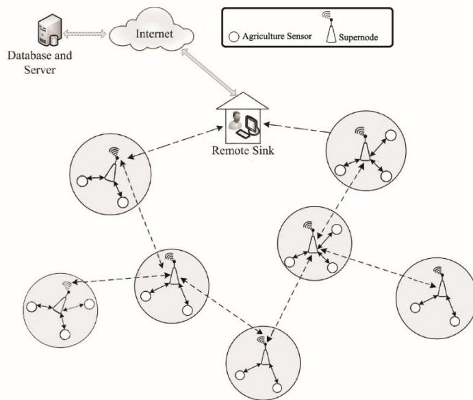
**Figure 1.** Smart agriculture based on heterogenous wireless sensor network.
