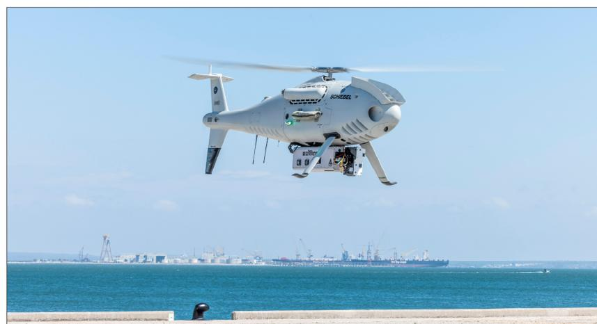
**Figure 3.** Schiebel CAMCOPTER® S-100 with Areté PILLS (RAMMS) LiDAR system [41].
