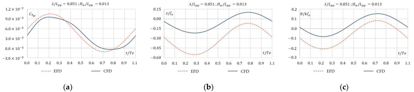
**Figure 6.** Comparison between CFD and EFD curves for (a) total resistance coefficient in wave amplitude, (b) heave amplitude, and (c) pitch amplitude for  $\lambda/L_{pp} = 0.851$  and  $H_w/L_{pp} = 0.013$ .
