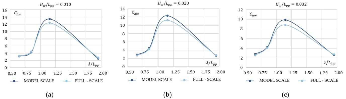
**Figure 9.** Comparison between model-scale and full-scale curves for wave added resistance coefficient in the case of (a)  $H_w/L_{pp} = 0.010$ , (b)  $H_w/L_{pp} = 0.020$ , and (c)  $H_w/L_{pp} = 0.032$ .
