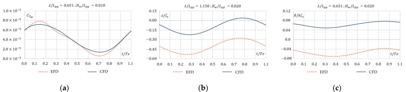
**Figure 5.** Comparison between CFD and EFD curves for (a) total resistance coefficient in wave amplitude, (b) heave amplitude, and (c) pitch amplitude for  $\lambda/L_{pp} = 0.651$  and  $H_w/L_{pp} = 0.010$ .
