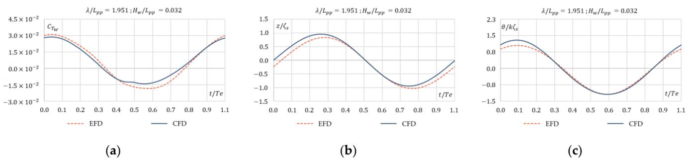
**Figure 8.** Comparison between CFD and EFD curves for (a) total resistance coefficient in wave amplitude, (b) heave amplitude, and (c) pitch amplitude for  $\lambda/L_{pp} = 1.951$  and  $H_w/L_{pp} = 0.032$ .
