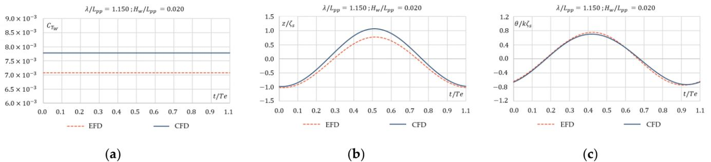
**Figure 7.** Comparison between CFD and EFD curves for (a) average total resistance coefficient in waves, (b) heave amplitude, and (c) pitch amplitude for  $\lambda/L_{pp} = 1.150$  and  $H_w/L_{pp} = 0.020$ .
