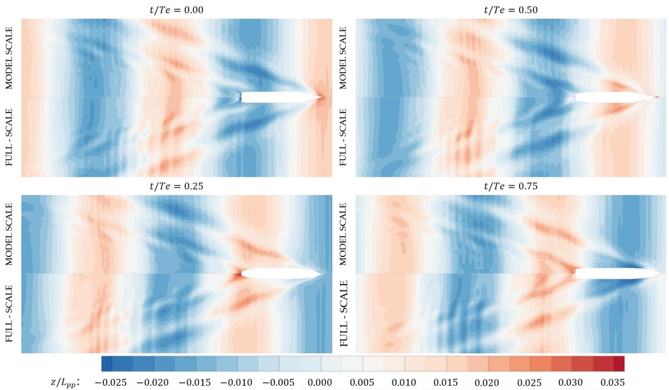
**Figure 13.** Comparison between model scale and full scale for wave elevation in regular head waves for  $\lambda/L_{pp} = 1.951$  and  $H_w/L_{pp} = 0.032$ .
