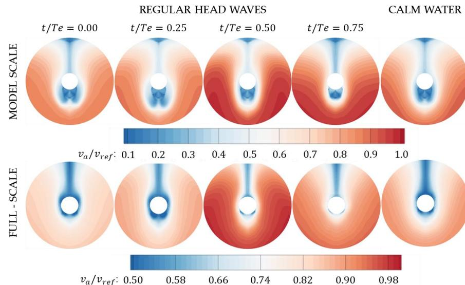
**Figure 15.** Comparison between model scale and full scale for axial velocity in the propeller in regular head waves for  $\lambda/L_{pp} = 1.951$  and  $H_w/L_{pp} = 0.032$ . Section at propeller plane.
