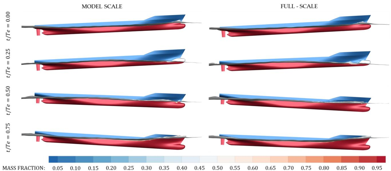
**Figure 14.** Comparison between model scale and full scale for mass fraction distribution in regular head waves for  $\lambda/L_{pp} = 1.951$  and  $H_w/L_{pp} = 0.032$ .
