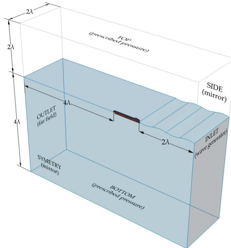
**Figure 2.** Computational domain and boundary conditions.
