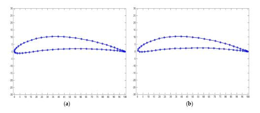
Figure 5. Optimized airfoil design using (a) SHO algorithm; (b) PSO algorithm.
