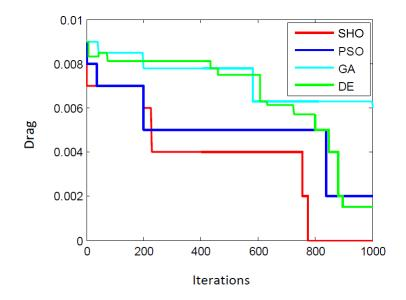
Figure 6. Convergence curves of airfoil design using SHO and other competitive approaches.
