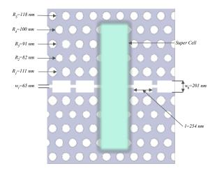
Figure 3. Optimized super cell using the SHO algorithm.
