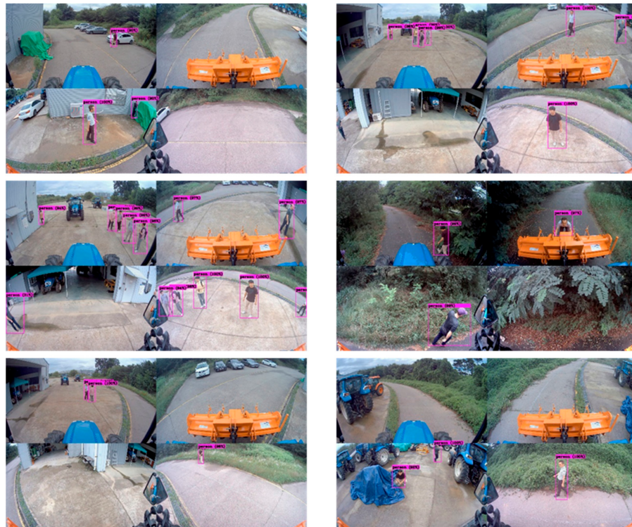
Figure 8. Person recognition test for autonomous tractor.
