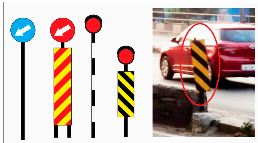
Figure 4. The multiple solutions seen on roads to show dividers. The current signage is displayed in the right part of the image within the red circle.
