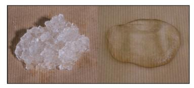
**Figure 1.** Visualization of superabsorbent polymers (SAPs): SAP<sub>CT</sub> (left) and SAP<sub>PT</sub> (right) containing absorbed water.
