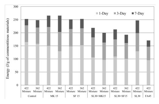
Figure 2. Heat of hydration of 422 and 363 mixture groups.
