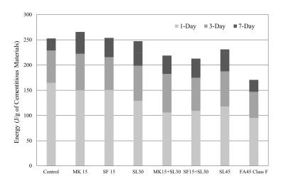
Figure 5. Heat of hydration of the 422 group mixtures.
