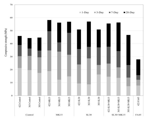
Figure 1. Compressive strength development of 422, 363, and 303 mixture groups.
