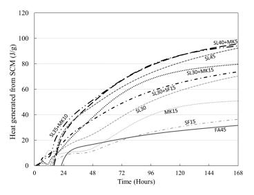
Figure 11. Heat of hydration generated from the pozzolanic reaction.
