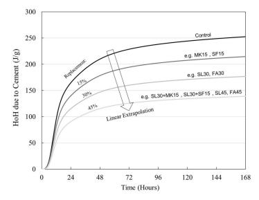
Figure 9. Linear extrapolation of the heat of hydration of the control mixture.
