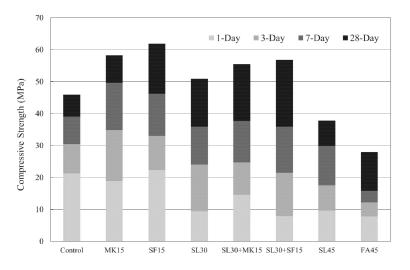
Figure 6. Compressive strength development of the 422 group mixtures.
