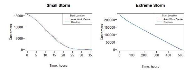
**Figure S1.** Start location for simulated small storms with 1,000 outages and extreme storms with 15,000 outages. Crew start location varied as indicated. Travel speed set to 25 mph, 272 crews with 85% working during day shift, 99% working during evening shift and 66% working during night shift, 1 to 10 hour repair time range and nearest outage search strategy. ETR curve was insensitive to crew start location.
