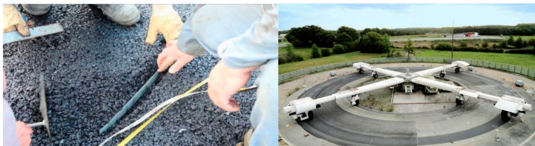
Figure 4. Installation of fiber optic cable at IFSTTAR accelerated pavement testing facility—pavement fatigue carousel (figures are reproduced from Chapeleau et al. [40]).
