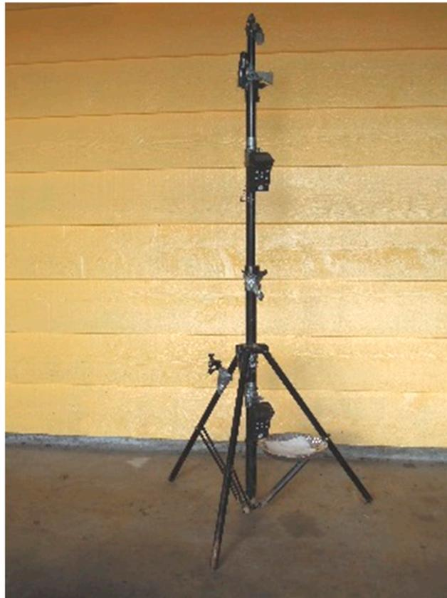
**Figure 1.** Equipment used to measure evaporation of solvent. Equipment included two instruments containing Photoionization Device (PID) sensors and two instruments for measuring temperature and humidity. The aluminum pie plate containing the paper towel onto which is poured the lacquer thinner is also visible.
