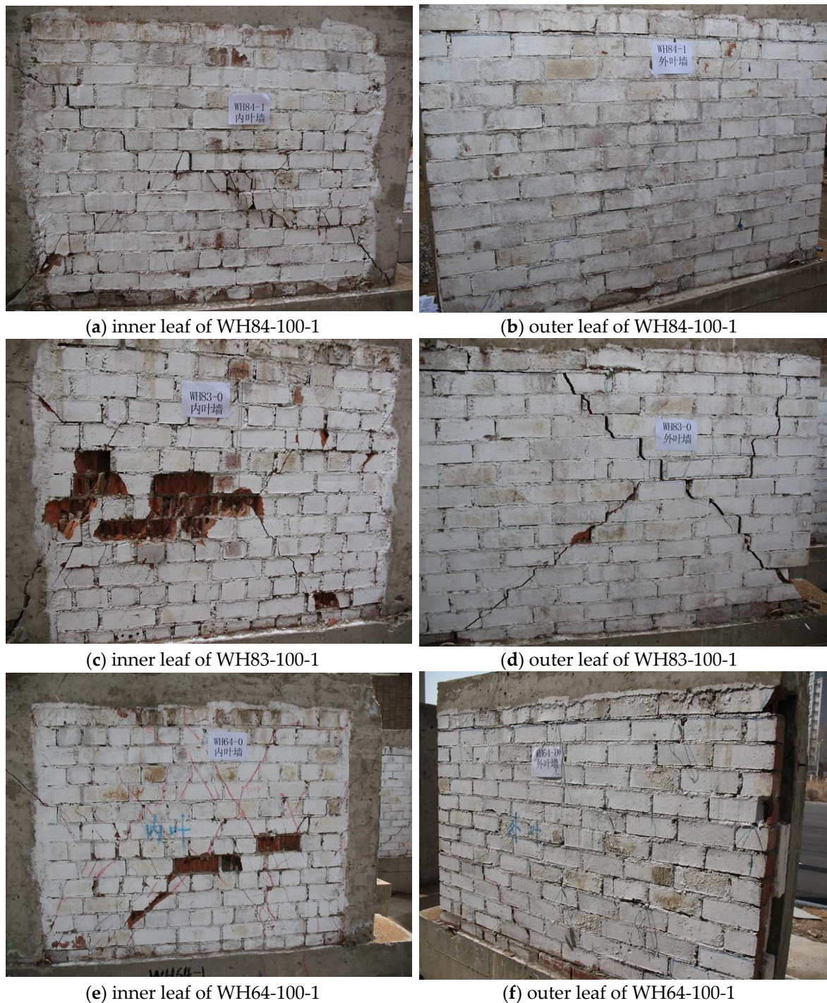
Figure 7. Damage state of the walls upon loading.
