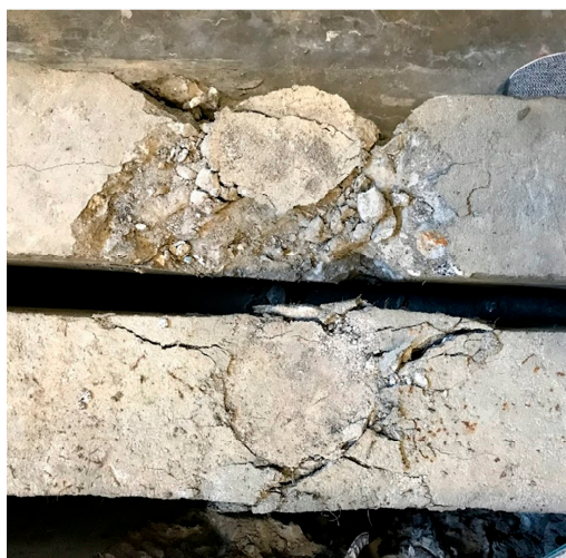
Figure 15. Top view of 40% PR (top) and Combination 2 (bottom) impact beams.
