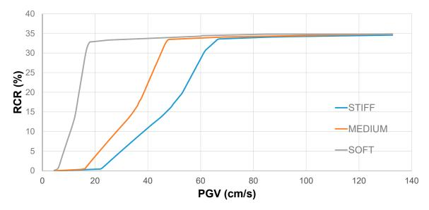
Figure 8. Repair cost ratio (RCR) for the selected soils.
