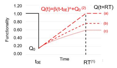
**Figure 6.** Proposed framework: (1) calculated by applying the performance-based earthquake engineering (PBEE) methodology; (2): recovery functions proposed in the present paper (parameters (a):  $\beta = 1$ ;  $\alpha = 1$ ; (b):  $\beta = 0.7$ ;  $\alpha = 0.85$ ; (c):  $\beta = 0.5$ ;  $\alpha = 0.75$ ).
