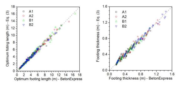
Figure 12. Optimum dimensions for retaining wall footing: Equation (3) vs. BetonExpress [27].
