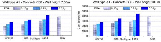
Figure 5. Cost of retaining walls type A1 made by reinforced concrete C30.
