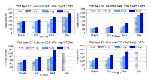
Figure 6. Cost of retaining walls type A2 made by reinforced concrete C25.
