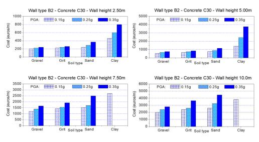
Figure 11. Cost of retaining walls type B2 made by reinforced concrete C30.
