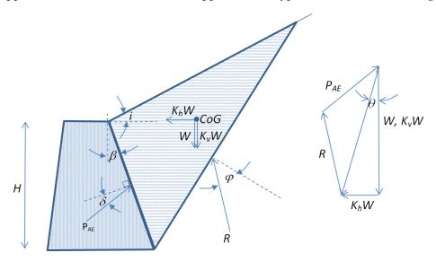
Figure 2. Stability checks for reinforced concrete retaining walls.
