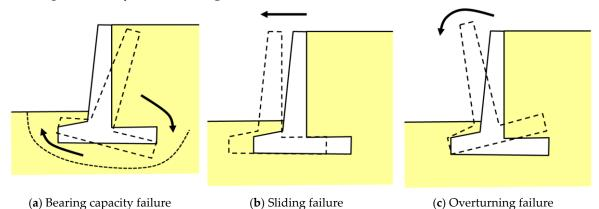
Figure 1. Stability checks for reinforced concrete retaining walls.
