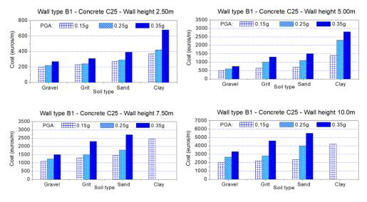
Figure 8. Cost of retaining walls type B1 made by reinforced concrete C25.
